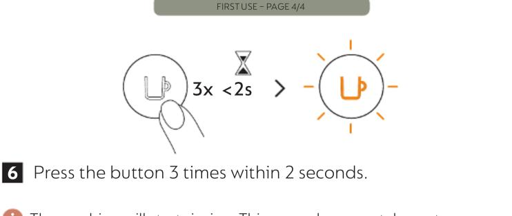
The machine will start rinsing. This procedure may take up to 7 minutes.
