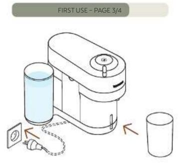
3 Plug the power cord, remove the cup support and place an empty container (at least 1 L / 34 oz) under the coffee outlet.
