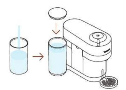
2 Fill the water tank with fresh potable water and put it back in position.
