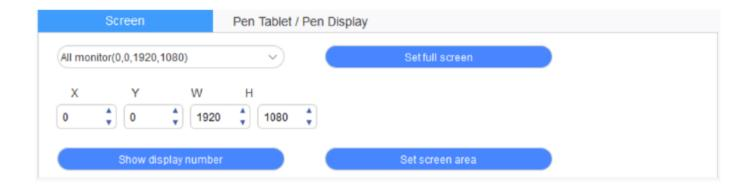
If multiple monitors are used in duplicate mode (i.e. All monitors display the same picture), the work area of the device will be mapped to all monitors. When the pen moves in the work area, the cursor on all monitors will move at the same time.
