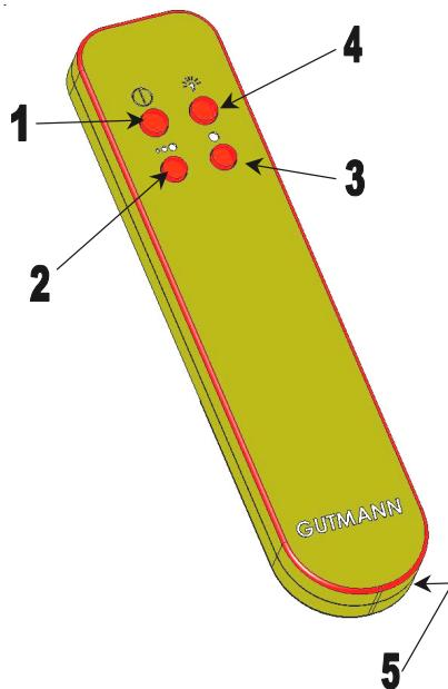
**Button 3:** Intensive stage (motor switches automatically back to Stage 3 after 3 min)
