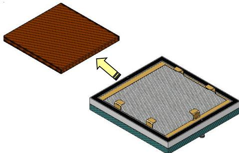
The active carbon filter is often mounted on a frame sitting below the ventilator module. For the exchange of the active carbon filter turn both black toggle screws around 90 degrees. After flapping down the pane and taking out the frame the filter can be changed easily. The installation is made in reverse order.
