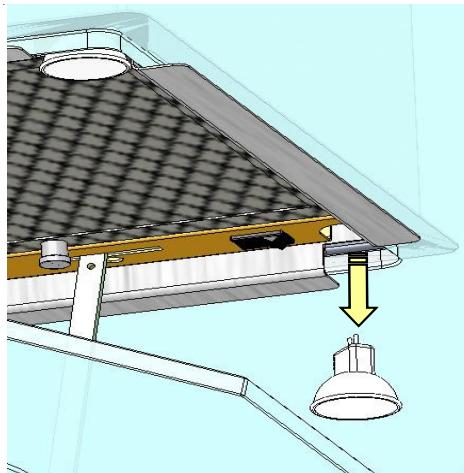
After cooling down, the illuminant must be held at the edge with both fingers, then move the illuminant down carefully (plug-in receptacle) until the illuminant is released from the socket. It is absolutely necessary to avoid contact with the skin during the insertion of the new illuminant; employ a clean cloth to do this. The installation of a new illuminant is
