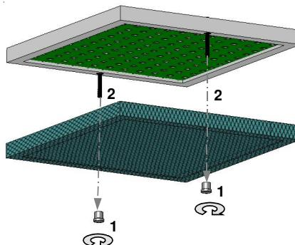
Before that, clean the metal filter parts where you screw off the filter grips for that. Now the metal filter can be disassembled into individual filter plates. The cleaning is best carried out in the dishwasher with a mild dishwasher cleaning agent.
