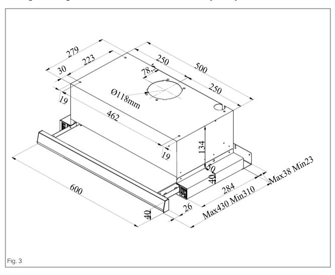
To achieve a flush fit with a decor door on the bridging unit, adjust the depth of the cutout by an amount equal to the difference between either 18 or 25.6mm and the thickness of the decor door. Please note that the canopy lip is shaped. The upper edge, which the decor door will meet, is 18mm thick.
