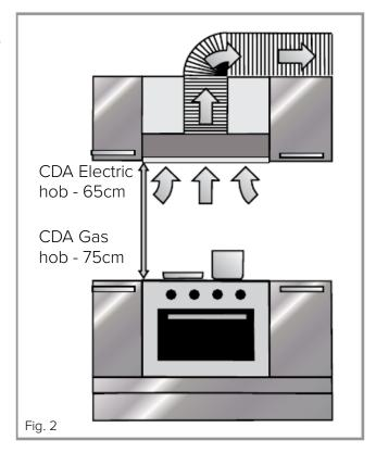
If the instructions provided with your gas hob state that the required distance between the hob and extractor must be greater than 750mm, then that is the distance that should be observed; this is a legal requirement and may lead to your hob being disconnected from the gas supply and the installation being reported under RIDDOR.
