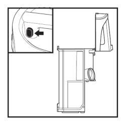
To remove collected debris from **Lint Screen**, press top release buttons either side of the handle and lift handle to access screen.
