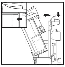
To remove **Dust Cup**, press release button on top of the pod. Tilt dust cup away from wand, then lift to remove.
