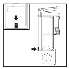
To empty debris into the bin, press lower release button and bottom of dust cup will drop open.
