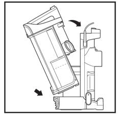
To reinstall, place bottom of dust cup into pod and then tilt until it clicks into place.
