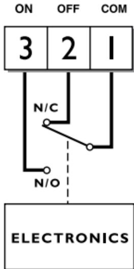
! Some existing thermostats will have a Neutral wire and/or Earth wire connected. These are not required by the TP4/5 and must NOT be connected to any TP4/5 terminals. Instead they should be made electrically safe and coiled in the recess at the back of the TP4/5.
