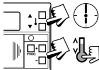
Press **PROG** until the colon in the LCD display starts to flash.
